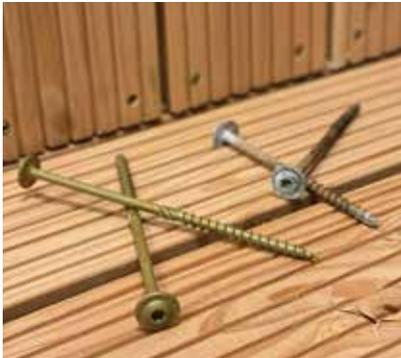
**DIFFERENCE BETWEEN AR COATING AND GALVANISED AFTER 6 MONTHS IN DOUGLAS-FIR WOOD**
